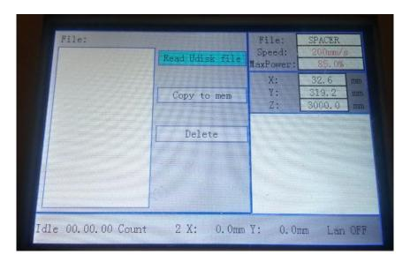
6.) Select the desired file and press enter on "Copy to mem". (Repeat this step for each desired file.)
