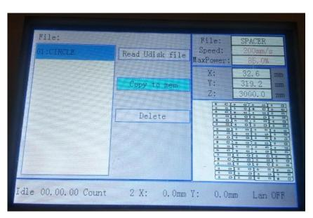
7.) Press "Esc" on the control panel to exit to the previous menu. The last file imported will appear at the top of the list while the rest will remain at the bottom of the list in the order they were imported.
