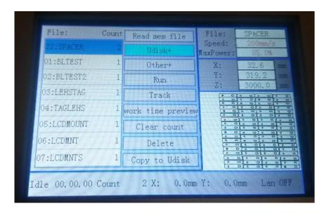
5.) Select "Read Udisk file" and press enter to read the files on the USB device.
